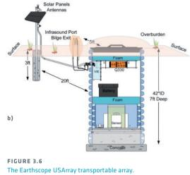
The Earthscope USArray transportable array. a) Status in April 2011. b) Schematic of a station installation including infrasound detector. From *Woodward et al.* (T3-012).
