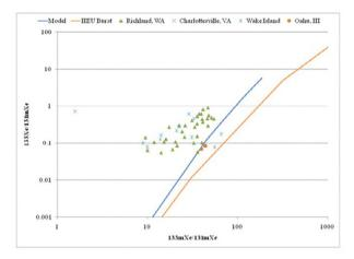
FIGURE 7.5 Comparison of xenon isotope ratios based on observations of the Fukushima accident at the IMS and non-IMS stations shown, together with discrimination lines. HEU refers to highly erriched uranium. From *Bowyer et al.* (JS-07).
