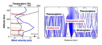
FIGURE 6.1 Acoustic ray tracing used to show the propagation of infrasound waves in the atmospheric waveguide formed by the temperature and wind variations in the different atmospheric layers. From *Blanc* (T1-01).
