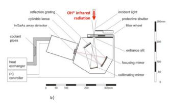
FIGURE 3.5 The Ground-based Infrared P-branch Spectrometer (GRIPS), for detecting infrared airglow. a) General view. b) Schematic. From *Bittner et al.* (T3-013).
